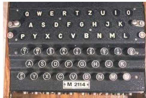
Figure 3. Keyboard and Lamp board[4].
