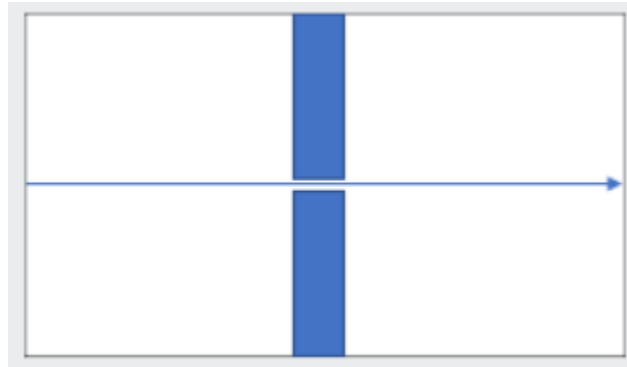
Figure 1. Light beam pass through the gap.
